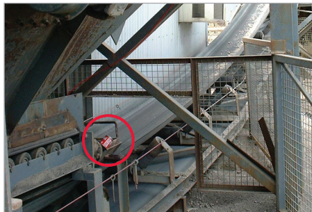
Lubrication of pillow block on a belt weigher
